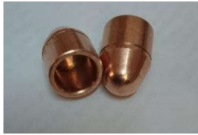
Fig 4.1: Photograph of Class 2 Copper Chromium electrode.
